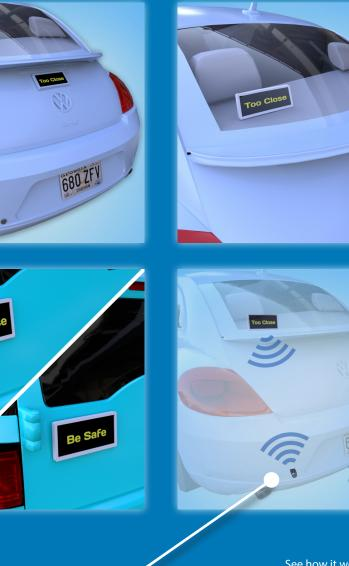
Sensor calculates speed and triggers the display in the window or back of car
